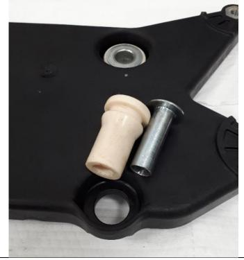
Insert grommets and standoffs into supplied ECM bracket.
