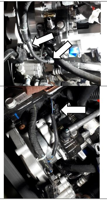
Ensure wiring is all secured and won't rub on hard parts.
