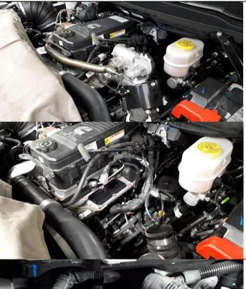
Remove nut from harness support, and remove CP4 support bracket from engine.
