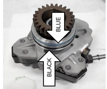
Set the correct timing for the pump as follows.
