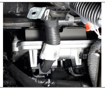
Install rail plug in most rearward feed port on fuel rail. Torque to specification.
