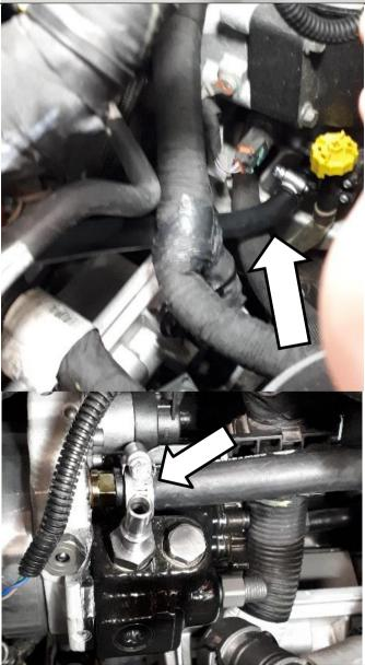
Connect OEM return hose to CP3 pump as shown.
