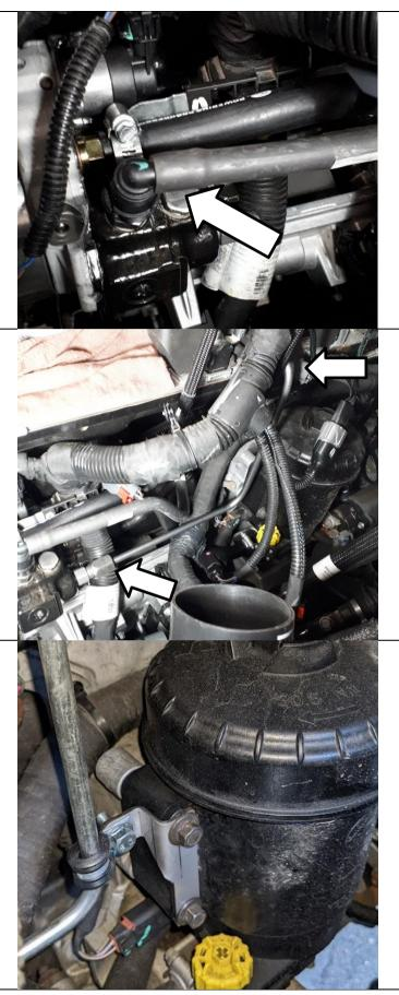
Remove factory loom 'Y'-clip, and both clips attached to the CP4 harness connector.
