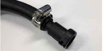
Remove factory feed hose from bottom of fuel bowl, and replace with ½" fuel hose assembled in previous step. Connect hose to CP3 pump inlet fitting with supplied clamp.
