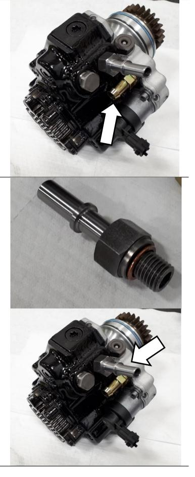
Remove OEM return fitting, and install supplied Quick-Connect fitting. Use supplied seal washer 1502019.
