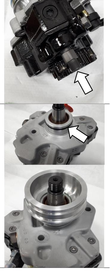
Ensure CP3 pump o-ring is installed, and install pump collar onto the front of the pump.
